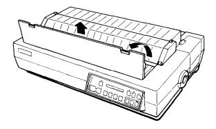
2. Open the paper guide cover as shown in the illustration. Then raise the cover slightly and lift the cover away from the printer at a slight upward angle.
